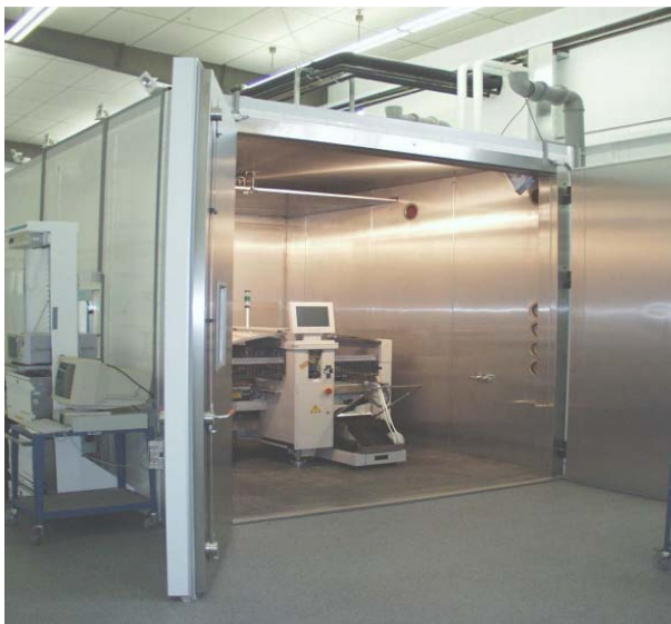
Pick-and-place system undergoing climatic testing
