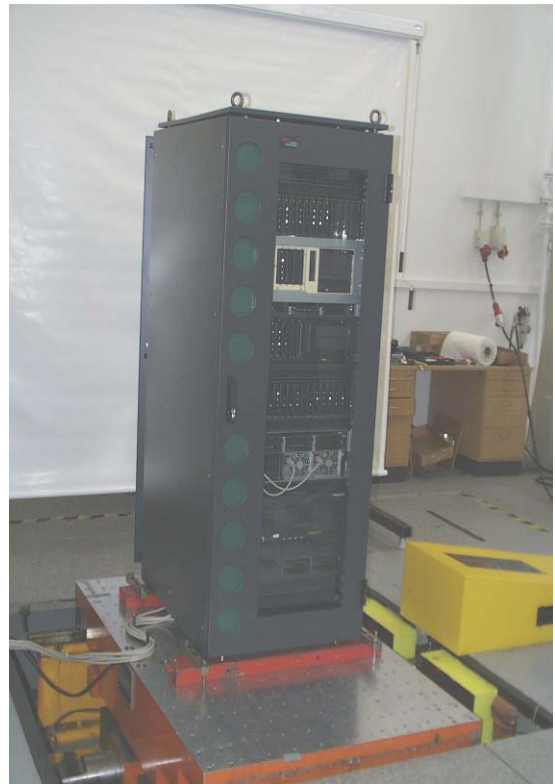
Earthquake test with IT equipment
